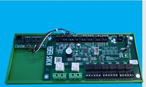
SimpleKey Event Manager (SEM) allows additional building functions to be controlled and monitored when connected to a SimpleKey system controller.
