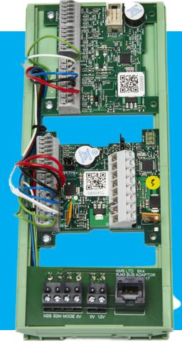
The SimpleKey 4 door extension kits allow additional doors to be controlled when connected to a SimpleKey 4 system controller. Available in one or two door versions, in a DIN rail format with simple connections to the free topography KMS Bus.
