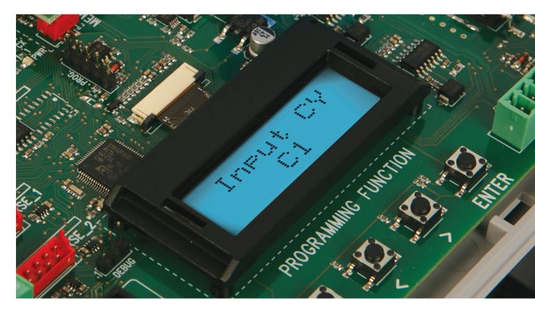
All BKV motors include a full graphical display to improve your experience when setting up the motor & performing maintenance.
