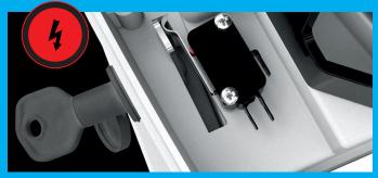
▲ THE POWER IS AUTOMATICALLY ISOLATED Unlocking the release door will automatically isolate the power.
