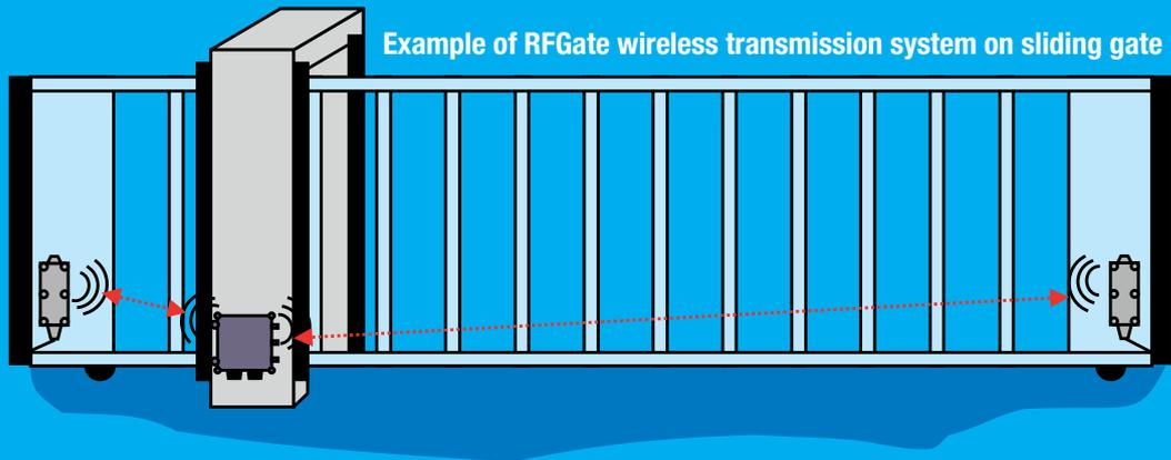
Example of RFGate wireless transmission system on sliding gate
